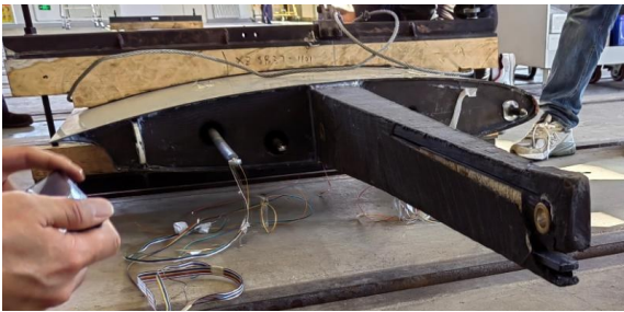
图5 拆卸机翼后的翼梁根部整体形貌 Fig. 5 The condition of the wing spar root after disassembling the wing
